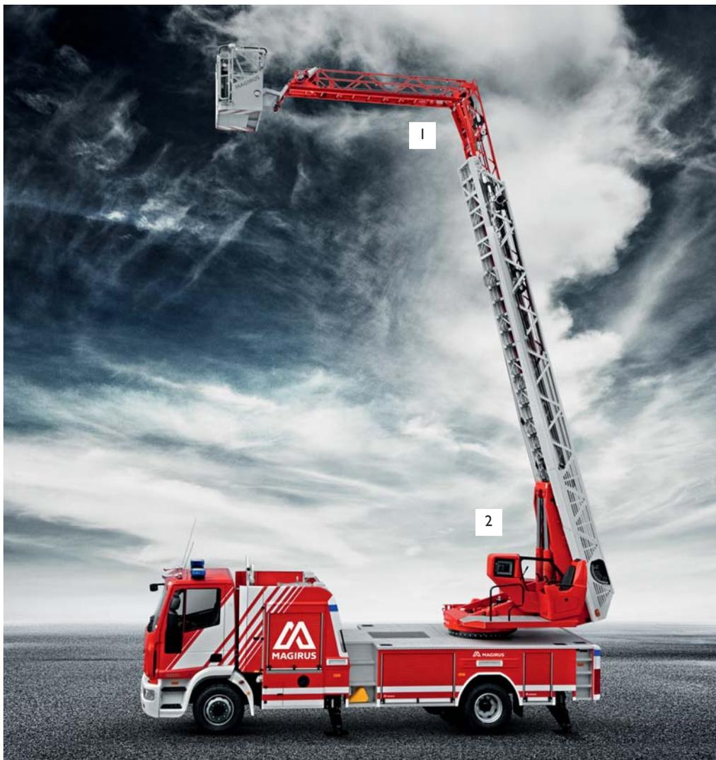
/ The top ladder section (1) and turning drive (2) of all Magirus turntable ladders are series equipped with anchor points for rope rescue and fall protection. (Certified anchor points for personal safety based on EN 795; protection for up to 500 kg / 2 people).
