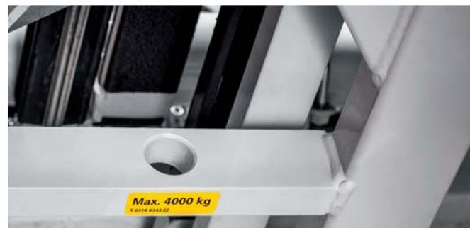
/ With the standard load eye at the lower ladder section, loads of up to 4000 kg can be moved (up/down/ turned).
